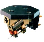
Te Kaitora is the result. A titanium headblock is used for lightness and rigid construction. The Te Kaitora has a 6mm solid boron cantilever fitted with a Pathfinder line contact stylus. The coils are wound out of very fine silver. A compliance of 10 CU and weight of 8.8 grams make it compatible with arms from Well Tempered, Linn, Naim, SME and others.
