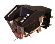
The XV-1s has a unique magnetic circuit. It comprises 8 small alnico magnets. The magnetic path is then divided into two. In the magnetic gap, a specially designed magnetic flux equalizing piece is the placed. On
