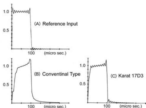
The effect of dispersion is shown by (A) is the input square waveform comprising harmonic frequency component up to 200th higher harmonic component. (B) shows the wave deformation by the dispersion in 7mm length conventional cantilever. (C) shows the effect of dispersion in 1.7mm cantilever of KARAT17D3. By shorter cantilever the smaller dispersion effect is recognized by these diagrams.
