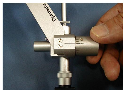
You will find whilst doing this that the mounting of the counterweight stub is flexible, this is deliberate and a feature that is designed to reduce resonances in the arm
