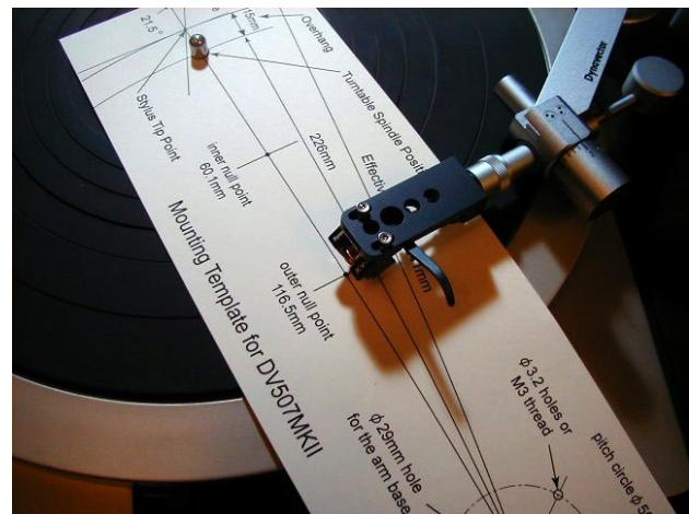
NOTE: You can easily check the overhang by using the mounting gauge supplied - see above, which fits between headshell and arm. When the stylus rests on the zero point then overhang is perfect. The inner null point and the outer null point on the mounting template is correct when the overhang alignment is set using this gauge.
