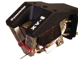
The XV-1s has a unique magnetic circuit. This comprises 8 small AL-NICO magnets. The magnetic path is then divided into two - In the magnetic gap, a specially designed magnetic flux equalizing piece is placed. Then on the
