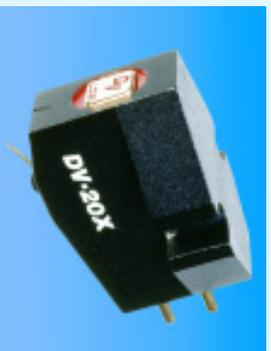
DV-20X has a solid aluminium-alloy body similar to the XX-2. The cantilever is a 6mm length of hard aluminium pipe with an elliptical stylus. This cantilever assembly is coupled to sets of coils in the 20XH
