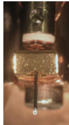
Dynavector showing the neat 8 coil array on special former showing fine workmanship
