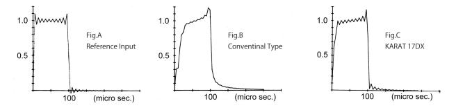
The effect of dispersion is shown by (A) is the input square waveform comprising harmonic frequency component up to 200th higher harmonic component. (B) shows the wave deformation by the dispersion in 7mm length conventional cantilever. (C) shows the effect of dispersion in 1.7mm cantilever of KARAT17DX. By shorter cantilever the smaller dispersion effect is recognized by these diagrams.
